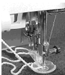
43 Freemotion couching foot Straight stitch • Attaching cords in a curved effect
